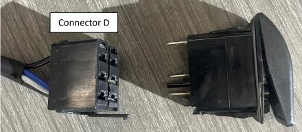
Remove the Rocker Switch(s) from Harness and NOTE THE POSITION OF EACH COLOR CABLE.
